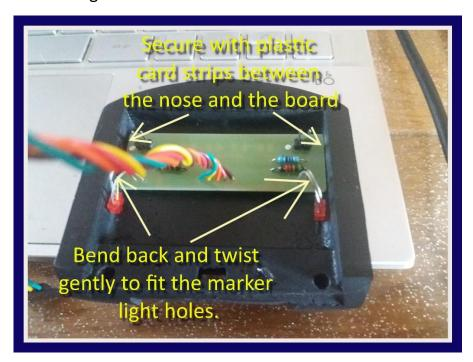
When happy with the test fit, use drops of canopy glue to fix the top-hat red marker lights in place. I add two strips of spare plastic card to each side of the nose lighting boards and, using small amount of superglue, also fix the board in place behind the head code recess in the nose.
