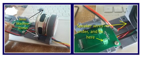
When you receive the ESU DCC Soundcard it will have a micro-speaker attached. Whilst it is not necessary to removed this, we do carefully unsolder the speaker because the 21-pin card sits better on the mounting plate "C" with the solder from these two fine wires removed.
