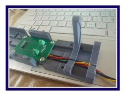
Next, secure the Fosworks speaker to the cradle mount supplied with your kit using two 3mm machine screws (do not overtighten). Make sure you align the speaker wires so that they neatly run the wires under the speaker through the notch in the 3d printed mount, and back towards the centre of the cradle mount. The wires will connect to the sound card mounting board which we'll address below.
